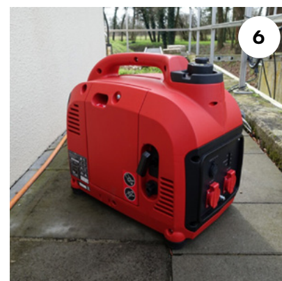
Switch on the generator according to the manual before plugging in the PSU or any other device
